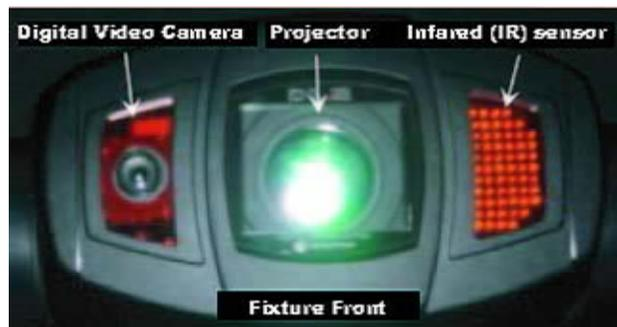
The DL.2 video camera is also equipped with an infrared (IR) illuminator sensor that makes it capable of "seeing" people and other subject matter in dark environments.
