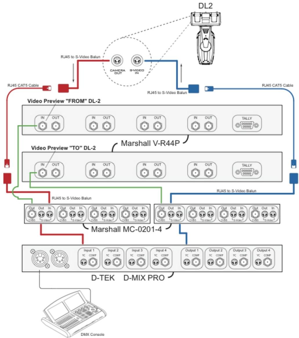
Example of how video preview monitors, S-Video to Composite converters and D-TEK Pro could be mounted in 1U rackmount configuration at FOH position
