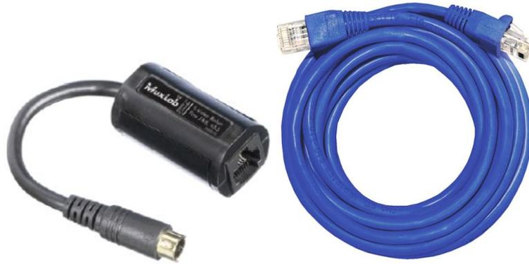
This longer distance should enable runs to front of house. MuxLab makes a video balun that does not require an external power supply. Two MuxLab 500016 S-Video baluns are required to send an S-Video signal from a DL.2 camera to the front of house using Cat 5 Ethernet twisted pair cable. The MuxLab S-Video baluns have a street price of about \$30 each.
